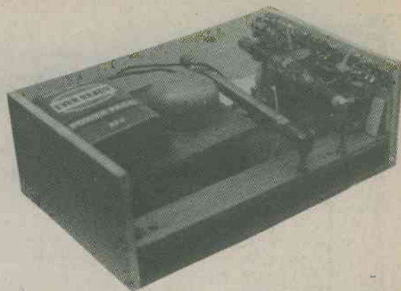
Side view showing details of the medium and long wave coil assemblies and the components on the 21-way tagstrip
